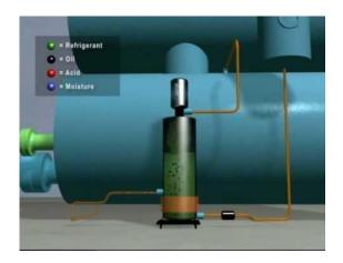
The OAM Purger operates non-stop as long as power is applied, whether or not the chiller is operating and cleans between 850 to 1250 pounds of contaminated refrigerant weekly.
